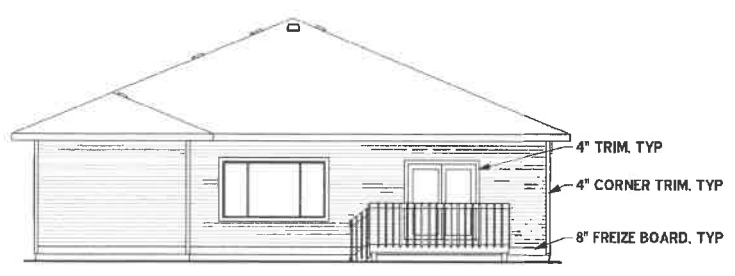
② Rear Elevation C - Mill Ridge 1/16" = 1'-0"
