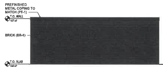
5 TRASH ENCLOSURE REAR ELEVATION 1/4" = 1'-0"
