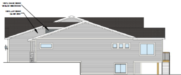
④ RIGHT ELEVATION - STREET VIEW 1/16" = 1'-0"
