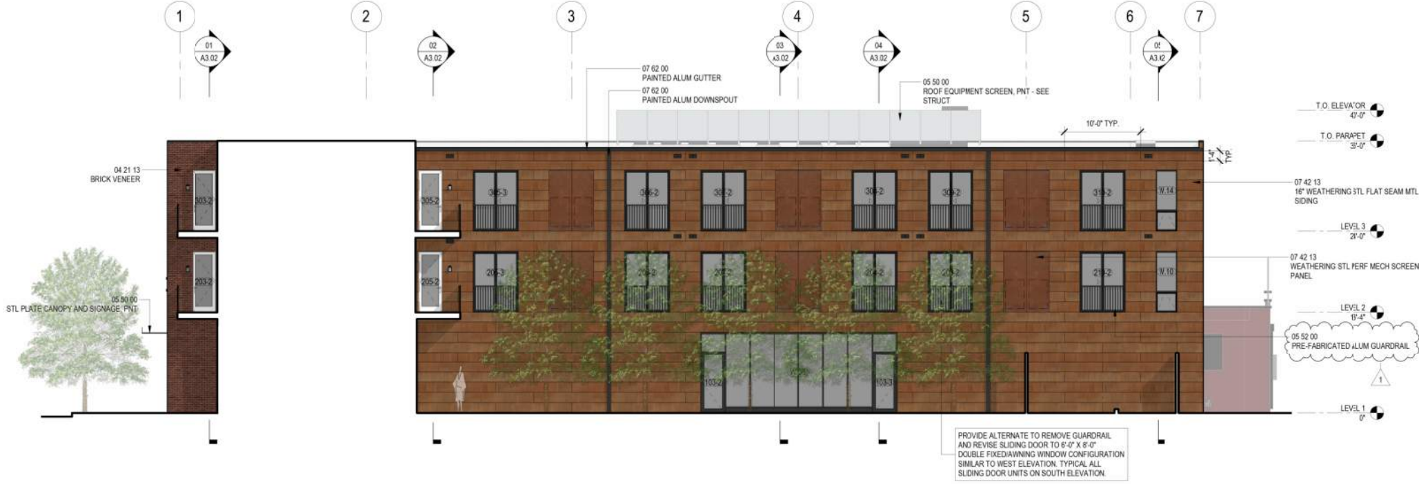
01 EXTERIOR ELEVATION - COURTYARD - NORTH SCALE: 1/8" = 1'-0"
