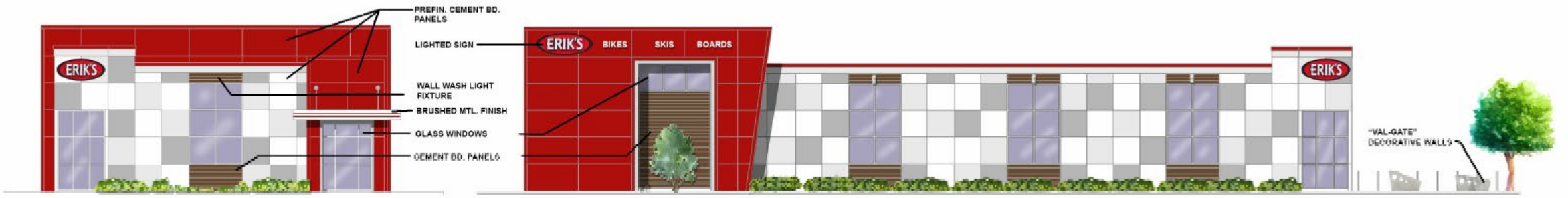
NORTH ELEVATION VIEW FROM ASHWORTH RD.
