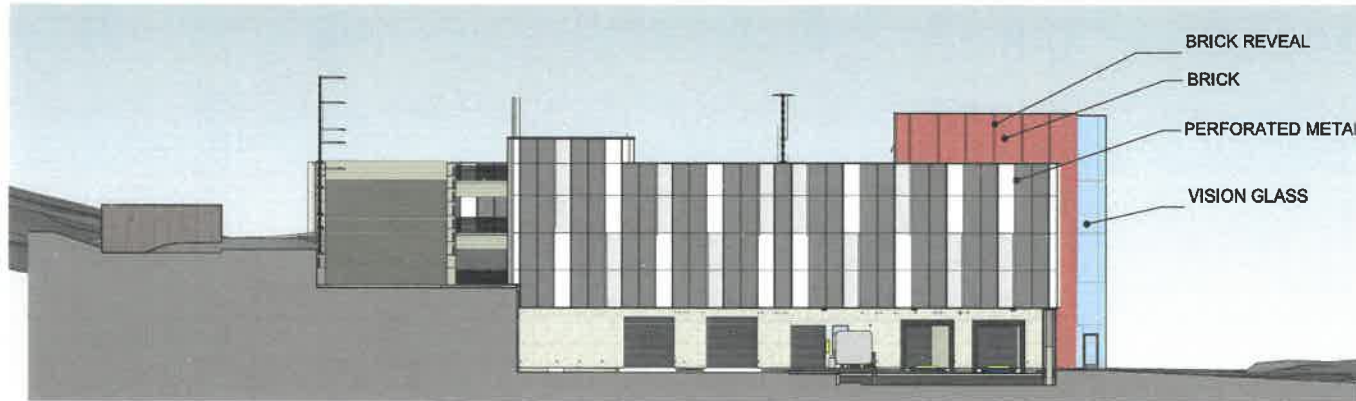
C1 EXTERIOR ELEVATION BLDG D WEST 1/8" = 1'-0" (A1/A1.D1)
