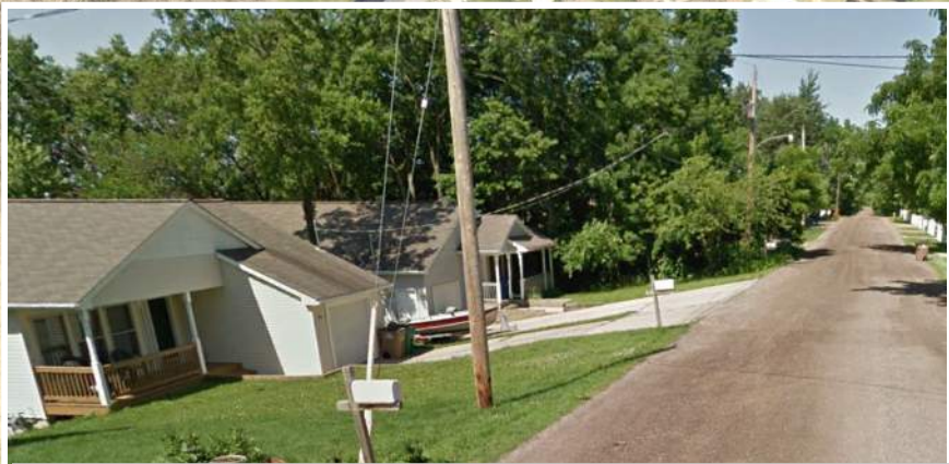
Several homes along the south side of High Street have driveways sloping steeply down from the roadway, causing a concern of flooding should curb and gutter be added channelizing flow in the roadway
