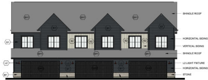
5C 3-PLEX GARAGE ELEVATION 1/8" = 1'-0"
