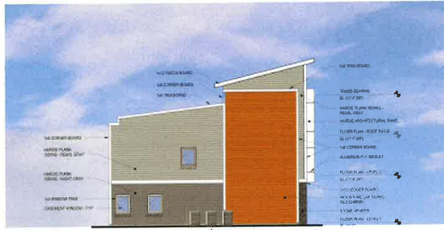
④ BUILDING 7 - LEFT ELEVATION
