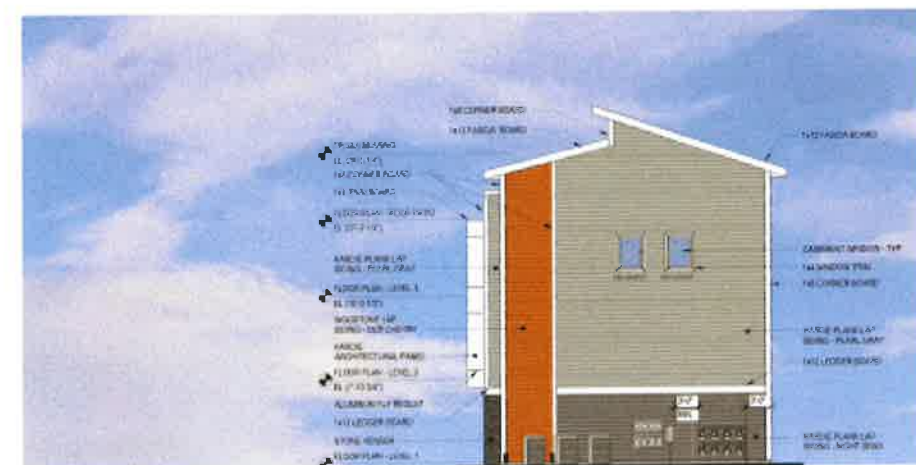
3 BUILDING 4 - THREE BEDROOM UNITS - RIGHT ELEVATION
