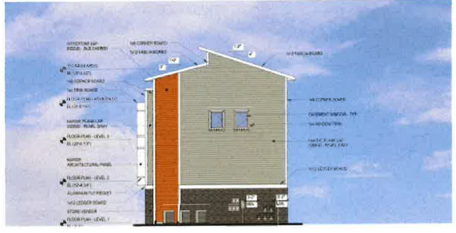
③ BUILDING 1 - THREE BEDROOM UNITS - RIGHT ELEVATION
