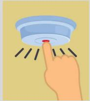
**REPLACE** – Replace all smoke alarms when they are 10 years old or stop responding when tested.
